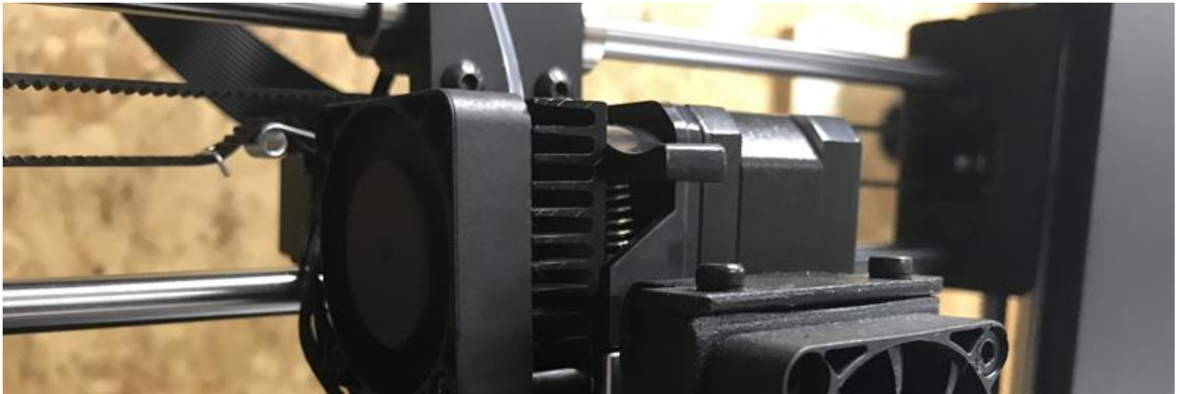
Example of a spring loaded direct drive
