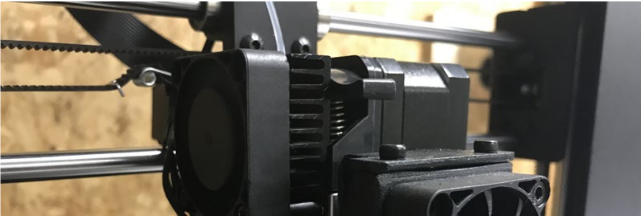
Example of a spring-loaded direct drive
