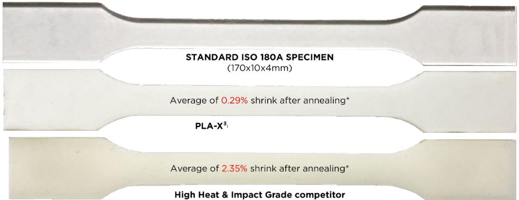
Specimens are printed at 50mm/s, 0.2 layer height, 0.4 nozzle, 100% infill and annealed in a pre-heated oven at 110c for 1 hour. After annealing the oven is allowed to slowly cool completely off for the best crystallization results.
